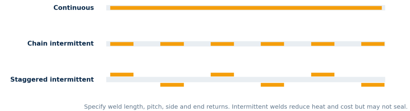
Figure 7. Continuous, chain-intermittent and staggered-intermittent concepts.
